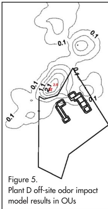
Figure 5. Plant D off-site odor impact model results in OUs
