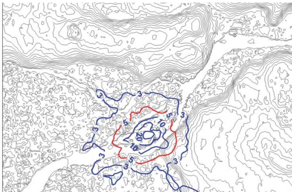
Figure 2. Plant A maximum predicted 10-min average odor concentrations (OUs)
