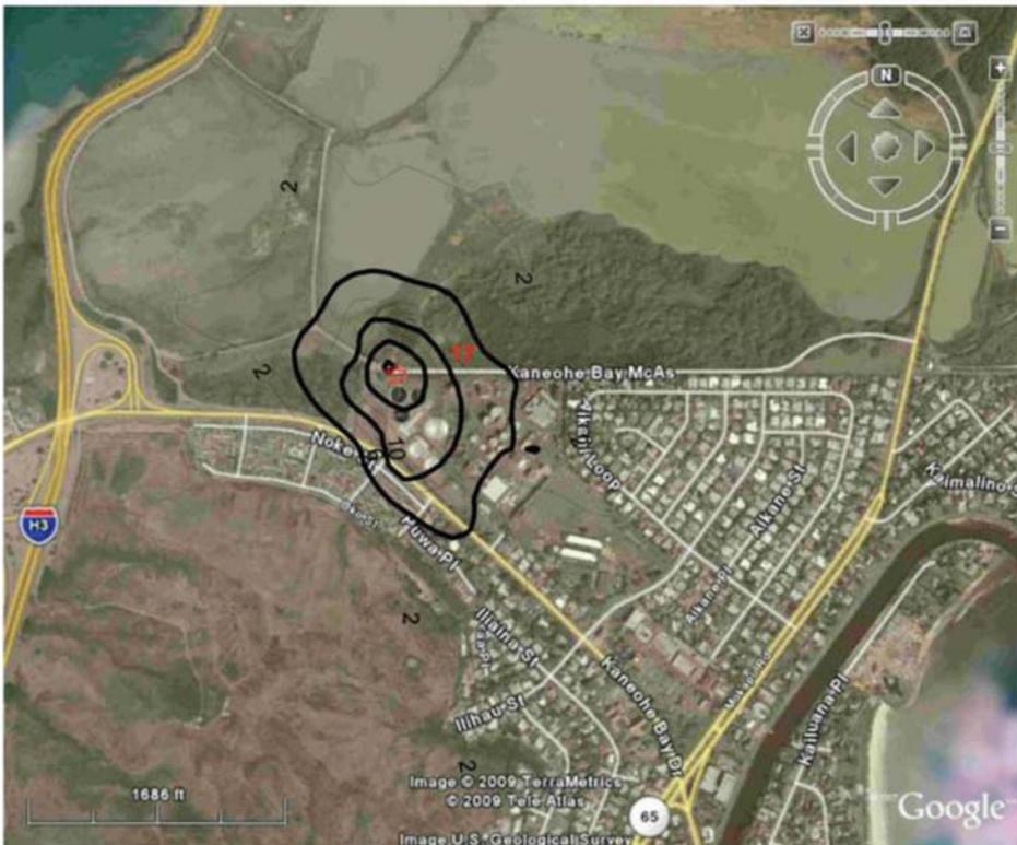
Figure 4. Plant C off-site odor impact model results in  $\mu g/m^3$   $H_2S$
