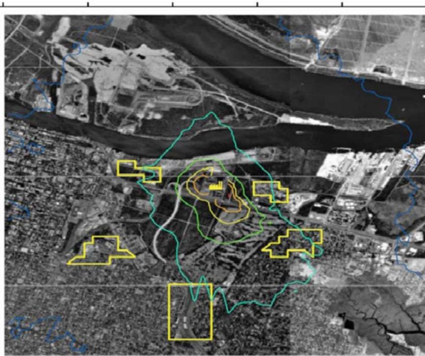
Figure 3. Plant B off-site odor impact model results in OUs
