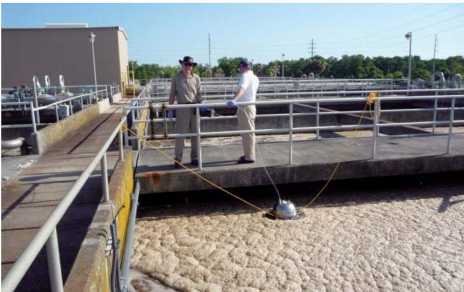
Figure 1. Flux chamber sampling
